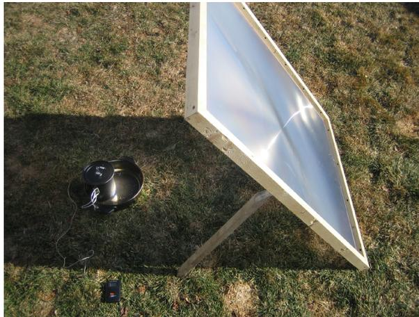
In this picture, you can see that I'm using a remote cooking thermometer. On an 18 degree day, it took 10 minutes and 28 seconds to heat the water from 58 degrees to 158 degrees. The lid being cracked made a BIG difference. The next time I did it, I didn't use a thermometer and the lid stayed closed. As a result, the temperature of the water was 177 degrees after 9 minutes. A few more minutes, and I would have had boiling water and I could have drawn off the steam and had distilled water.
